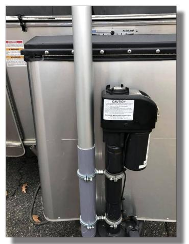
This is how we installed the extendable flag pole to our Airstream jack using pairs of clamps connected by stainless steel rods. This is very efficient way to mount the antenna and can be installed or repacked within three minutes.
