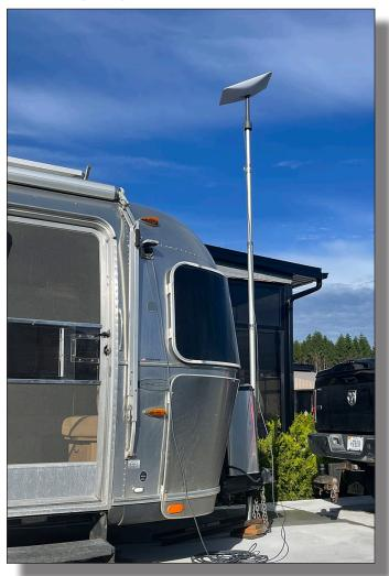
Campground installation near Quebec City with the flagpole extended to some 15 feet, enough to get the Dishy well clear of the surrounding buildings. Shows the cable route through the Furrion port to the router inside. Some Airstream Starlink users keep the router in an outside storage compartment and connect by Wi-Fi.
