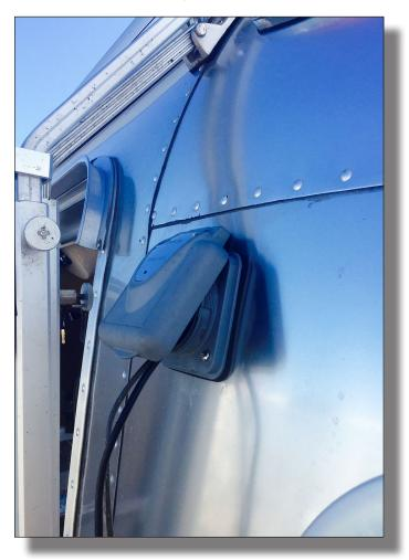
Cables to the Dishy antenna run through a modified Furrion shorepower port that we installed adjacent to the main door. We installed the cable port some years ago to be used for cables from the cellular booster and for the Wi-Fi booster antenna.
