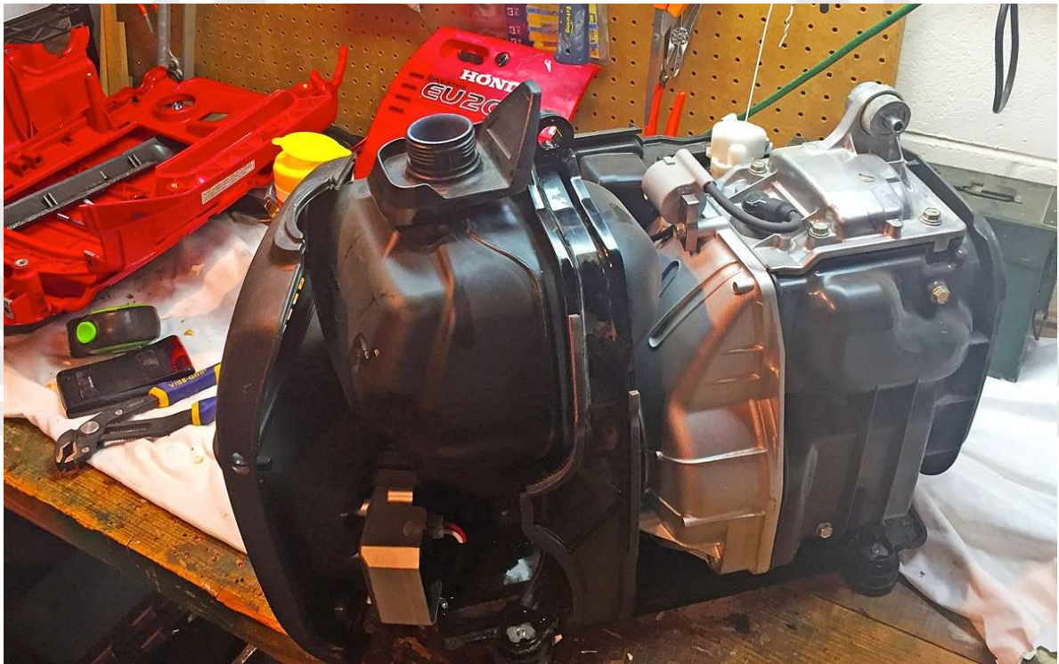
Honda Generator Propane Conversion (#28) Replacing the fuel tank and gas carb with propane regulator and propane carb kit from Genconnex Direct
