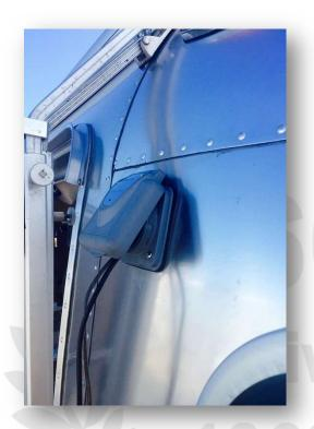
Cables to the Dishy antenna run through a modified Furrion shorepower port that we installed adjacent to the main door.
