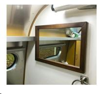
bathroom sink. Used recessed key hole hangers but also opted for a small central white polyester block (virtually invisible!) along the top edge of the frame to prevent Louisiana I-10 shake rattle and jump off the wall action!
