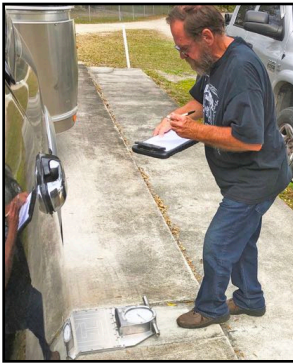
John Hamilton, Escapee weighmaster, records each scale reading onto the data sheet for the rig.
