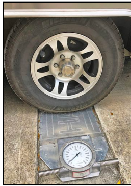
A pair of scales are used, one on each side of the rig. These highly accurate devices are recessed level into the concrete weighing platform so that no variations are introduced in the weighing process.
