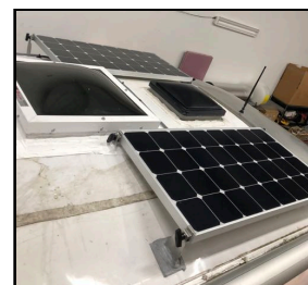
Four 100 watt solar panels installed on the roof of our Airstream, 2 forward and 2 in the rear.
