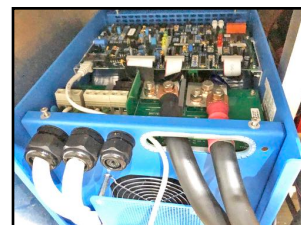
The inverter under the dinette berth - input 12volt black cables from batteries on the right, incoming shore power and outgoing 120 volt to distribution panel on left.
