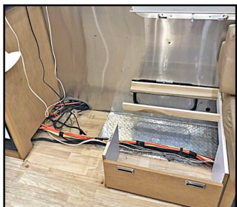
Removal of berth slide-out and inverter, and truncating the base frame.
