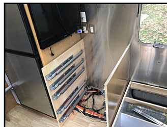
Addition of Blum slides to the end panels
