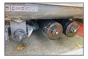
One special project we had DJ address was to add eight foot storage tubes under the rear of the Airstream which he designed, fabricated the fittings and installed.
