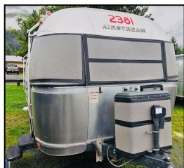
Vulnerable surfaces on the Airstream are protected against road debris using yoga mat material and Gorilla tape.
